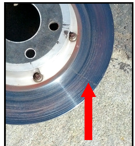
Arrow points to crack in the rotor. Photo by Larry Mason
